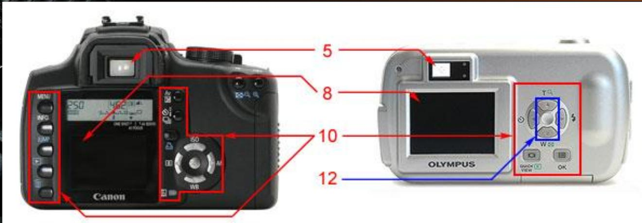
**10. Control Buttons** - Usually includes a set of directional keys and a few other buttons to activate certain functions and menus, this is used to let users interact with the camera's computer system.
