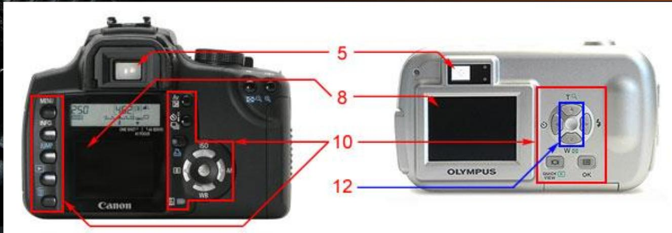
5. **Viewfinder** - A small viewing window that shows the image that the camera's imaging sensor sees. This can either be an optical view finder, which shows the actual image in front of the camera through a peep hole or through mirrors, or an electronic view finder which is simply a small LCD display.
