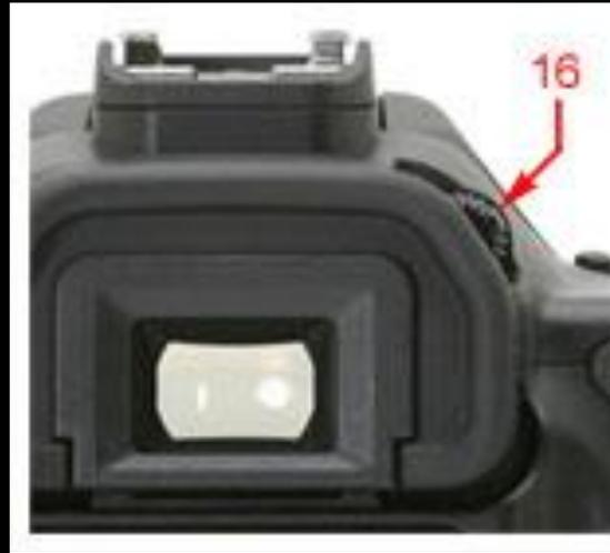
**16. Diopter Adjuster** - Usually available in mid to high end sub-compact cameras and DSLRs located besides the viewfinder. This varies the focal length of the lens in the viewfinder to make even people wearing eyeglasses to see clearly through it even without the eyeglasses.
