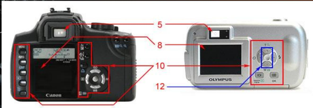
**8. LCD Display** - In some compact cameras this acts as the viewfinder. This is a small screen (usually 1.8" diagonally or bigger) at the back of the camera which can be used for framing or for reviewing the recorded pictures.
