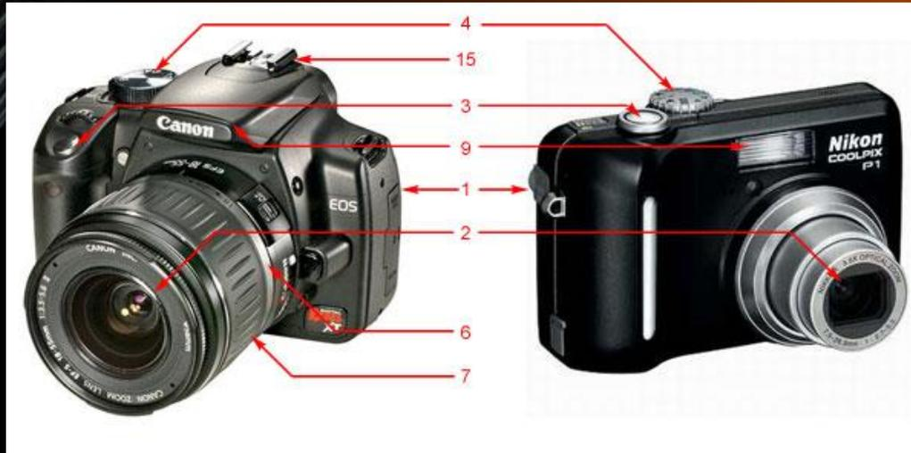
9. **Flash** - Built-in on the body of most compact and some DSLR cameras this can either be fixed or flip type, it provides an instantaneous burst of bright light to illuminate a poorly lit scene.
