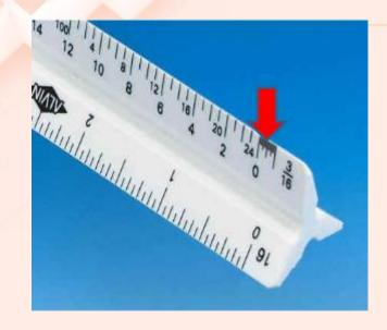
Each of these measurements on the architectural ruler is equal to 1' 3" in real life.
