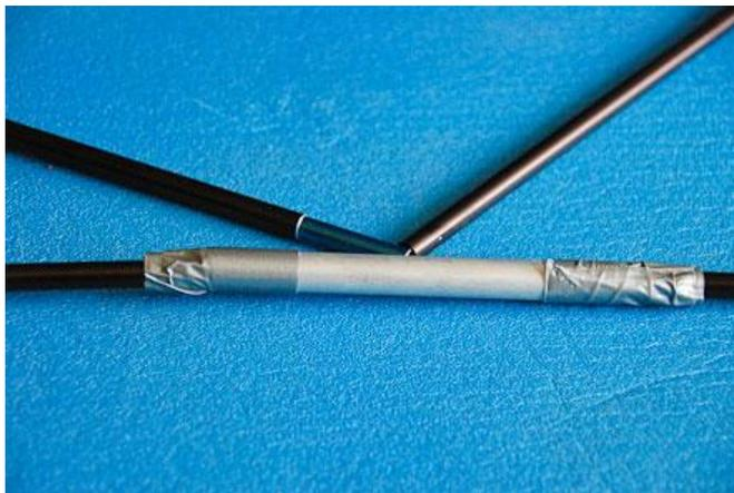
7. For a stronger, multi-night repair, mark where the repair sleeve sits when centered over the break.
