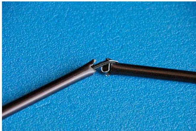
3. For a quick midnight repair, slide the repair sleeve over the broken pole section keeping it centered on the break.
