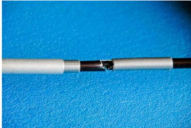
11. So it looks like this. If the tape fits tightly, you won't need to hold it in place with additional tape wraps. You can remove and reposition the repair tube at will for more efficient packing.
