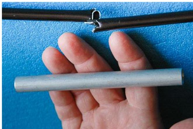
4. Notice how the broken pole ends have been rounded and cleaned up so they'll fit in the tube.
