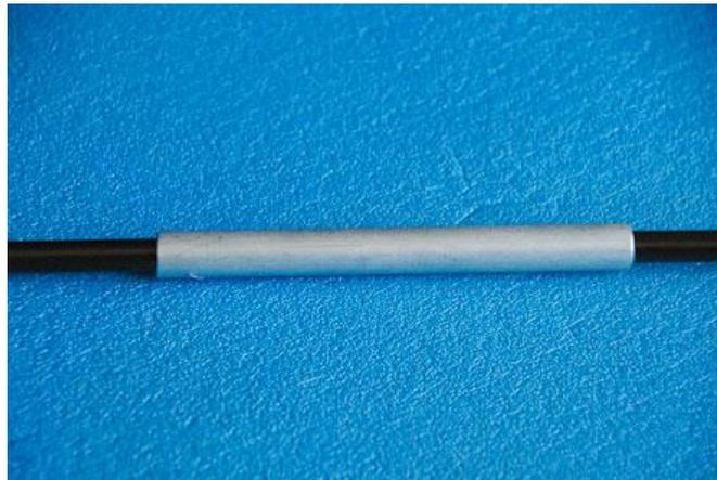
12. Why it's important. With both broken halves wrapped and fit tightly to the repair tube, the pole arc bends evenly with no pressure points that can fold again in high winds.
