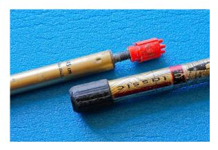
2. To solve the problem, first pull the pole apart and clean dirt and corrosion off the screw threads using a clean cloth or old toothbrush.
