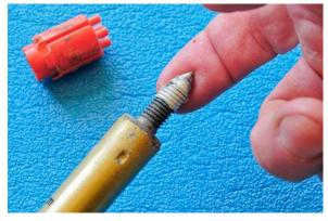
4. Then sand the plug's exterior to clean off any gunk and increase friction against the pole shaft interior by creating horizontal striations. For trail repairs you can use almost anything, even sand or pebbles.
