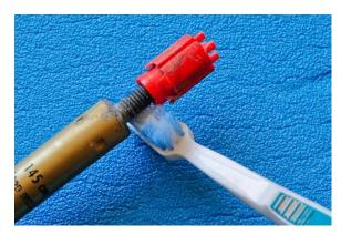
3. Lubricate the threads very lightly using bicycle grease, chapstick, or other non-running lubricant. DO NOT use WD40 or oil, since it will run onto the plug and pole interior over time, making the adjustment slip.
