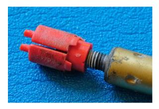
6. If the pole adjustment still slips, clean and roughen the interior of the female pole shaft. Here a hydration tube brush has been bent to match the wider pole circumference.
