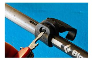
11. If the pole still slips, sand the interior of the compression collar and, if necessary, lightly sand the exterior of the lower, male-end pole.
