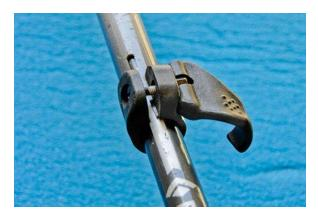
10. First step: Tighten the adjustment screw. If necessary, keep it from constantly loosening using LockTite.
