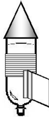
Look at your fin. Make sure it doesn't curve or it isn't crooked. It should be in a direct line with the body of your rocket. If it isn't perfect, take it off and try again. Attach the other fins. Test the wiggle of the fins. Your fins shouldn't wiggle more than a few centimeters from side to side. Adding more tape to the top and bottom areas of the fin might fix this problem.
