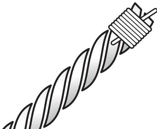
Slide the rope off the tools and let it relax a bit, whip or backsplice the ends (tape works temporarily) and you're done. Burn off the hairy fibers with a candle or propane torch if you wish.
