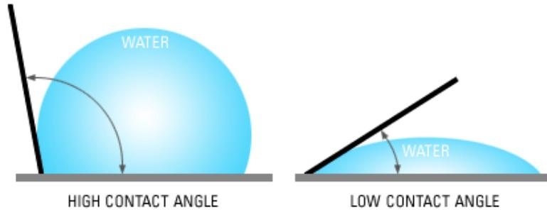
An optimized DWR keeps droplets in a rounder shape—like a dome-shaped bead. The rounder the droplet, the easier it rolls off the fabric. A low contact angle permits droplets to assume a flatter shape, one that can spread out like a splotch, cling to the fabric's surface and eventually seep into it.
