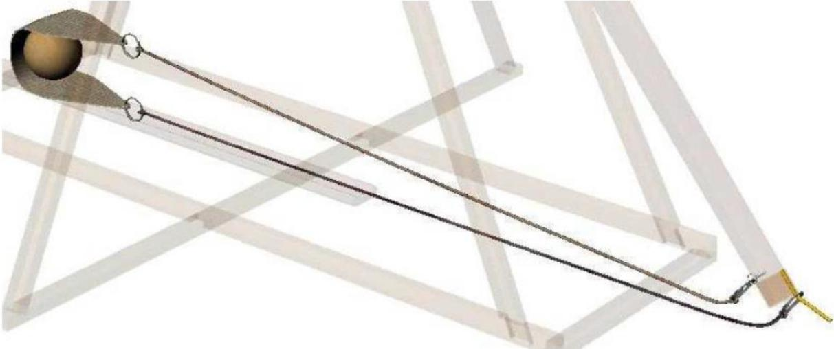
**Firing Pin/Trigger Mechanism for Trebuchet**
