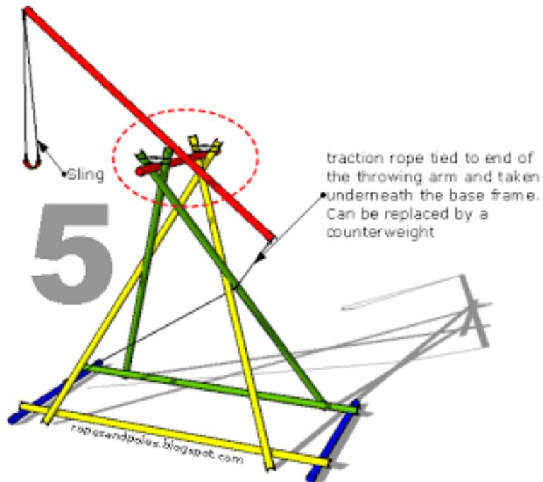
**Replace traction rope with a counterweight**
