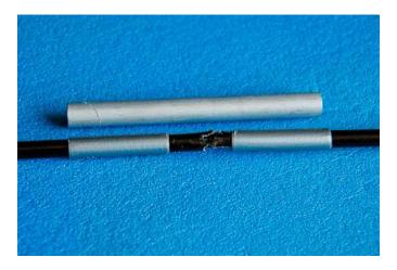
10. Slide the repair tube over the duct taped pole section.
