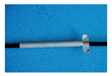
8. Wrap one broken end with duct tape so that it fits tightly into the sleeve and the tape goes all the way to the end of the repair tube's length. Position the tube and mark the opposite end.
