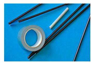
2. A broken aluminum pole will usually crimp and shatter. If necessary, break off metal shreds and squeeze the flattened ends until they fit into the repair sleeve. Fiberglass poles generally fray but stay connected. Repair procedures are the same.
