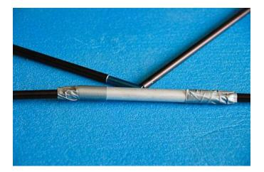
7. For a stronger, multi-night repair, mark where the repair sleeve sits when centered over the break.
