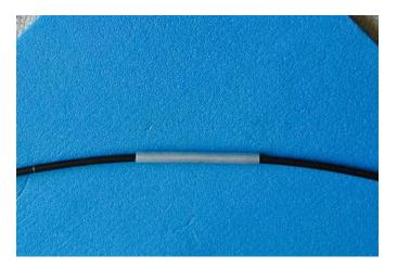
13. Why it's important. With a simple repair tube and no underlying duct tape wraps, the pole bends unevenly and the black pole sections are bent over the sharp edge of the repair tube, forming a weak point.
