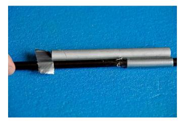
9. Wrap the other half of the broken end in similar fashion. Note how the two duct tape wraps go all the way to the repair tube ends.
